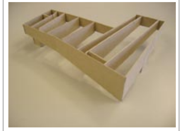
Support structure - first attempt Exploring the use of the facades and the cross walls as a support structure.
